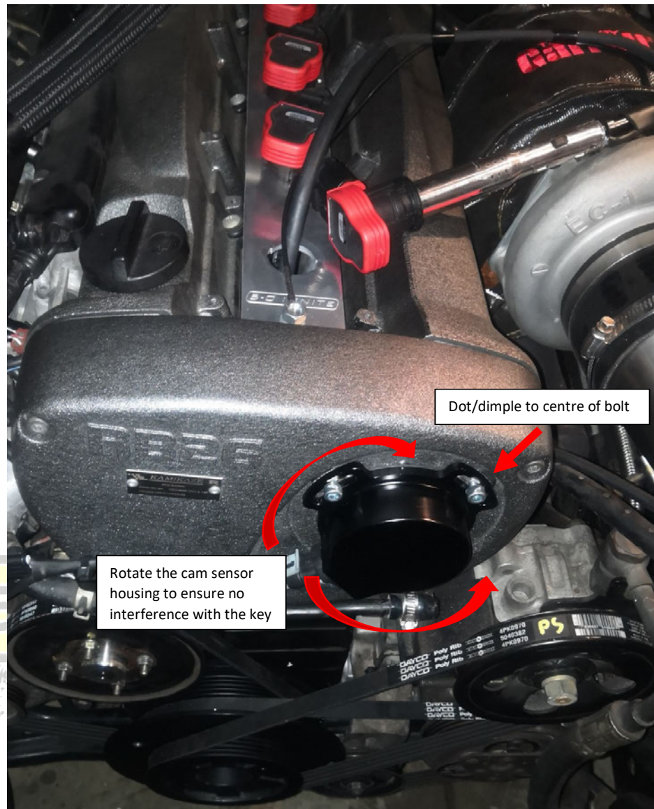
Figure 7 - Cam Sensor Housing Position
