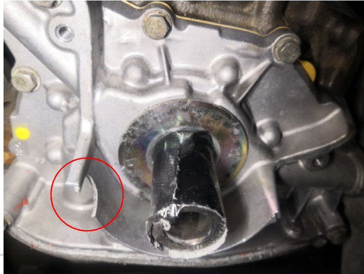
Figure 2 - Grind Slot on Oil Pump Housing
